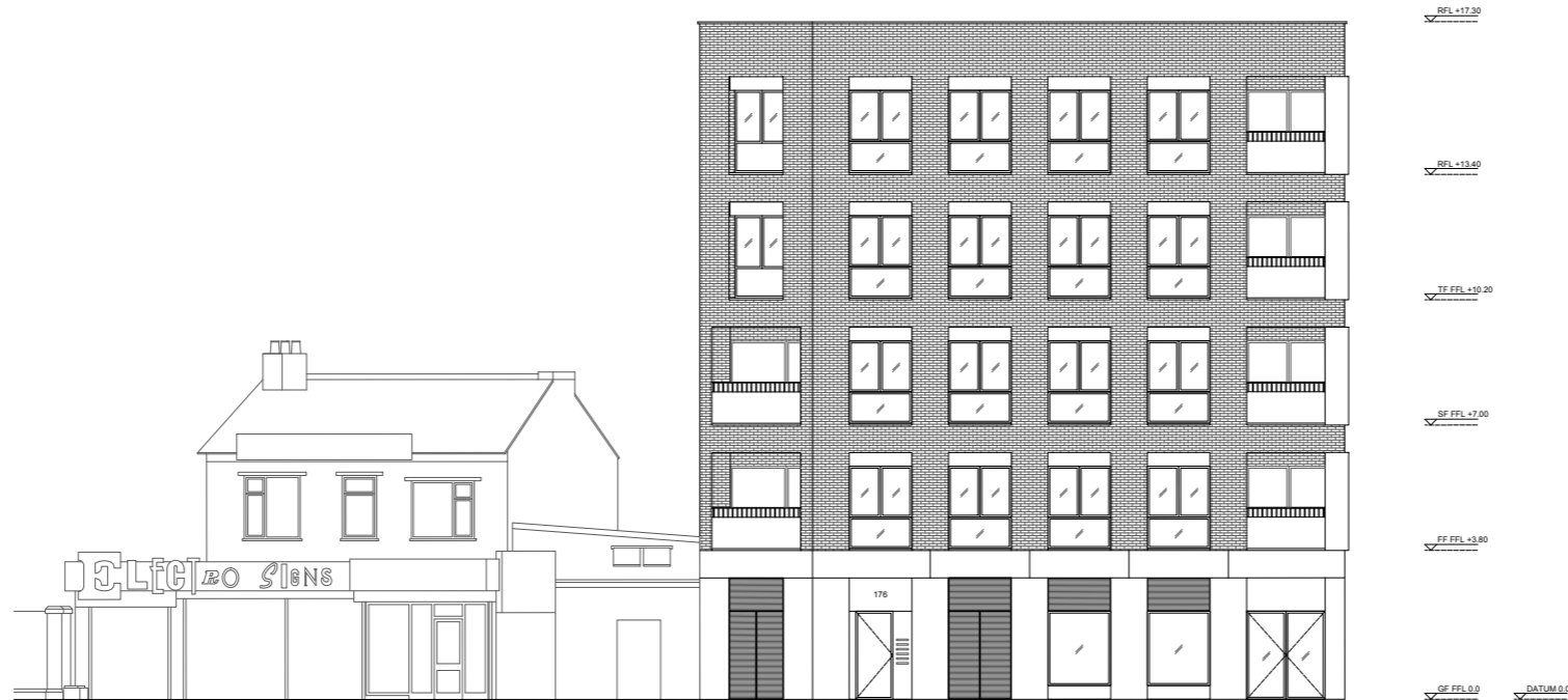
3 PROPOSED EXTERNAL ELEVATION - VALLENTIN ROAD Scale 1:100
