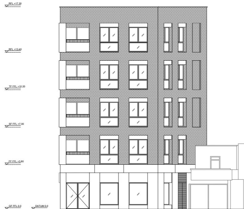
1 PROPOSED EXTERNAL ELEVATION - WOOD STREET EAST Scale 1:100
