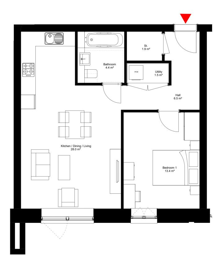
Proposed Dwelling Type - P1204 1:50 The contractor is responsible for checking dimensions, tolerances and references. Any discrepancy to be verified with the Architect before proceeding with the works. Where an item is covered by drawings to different scales the larger scale drawing is to be worked to.
