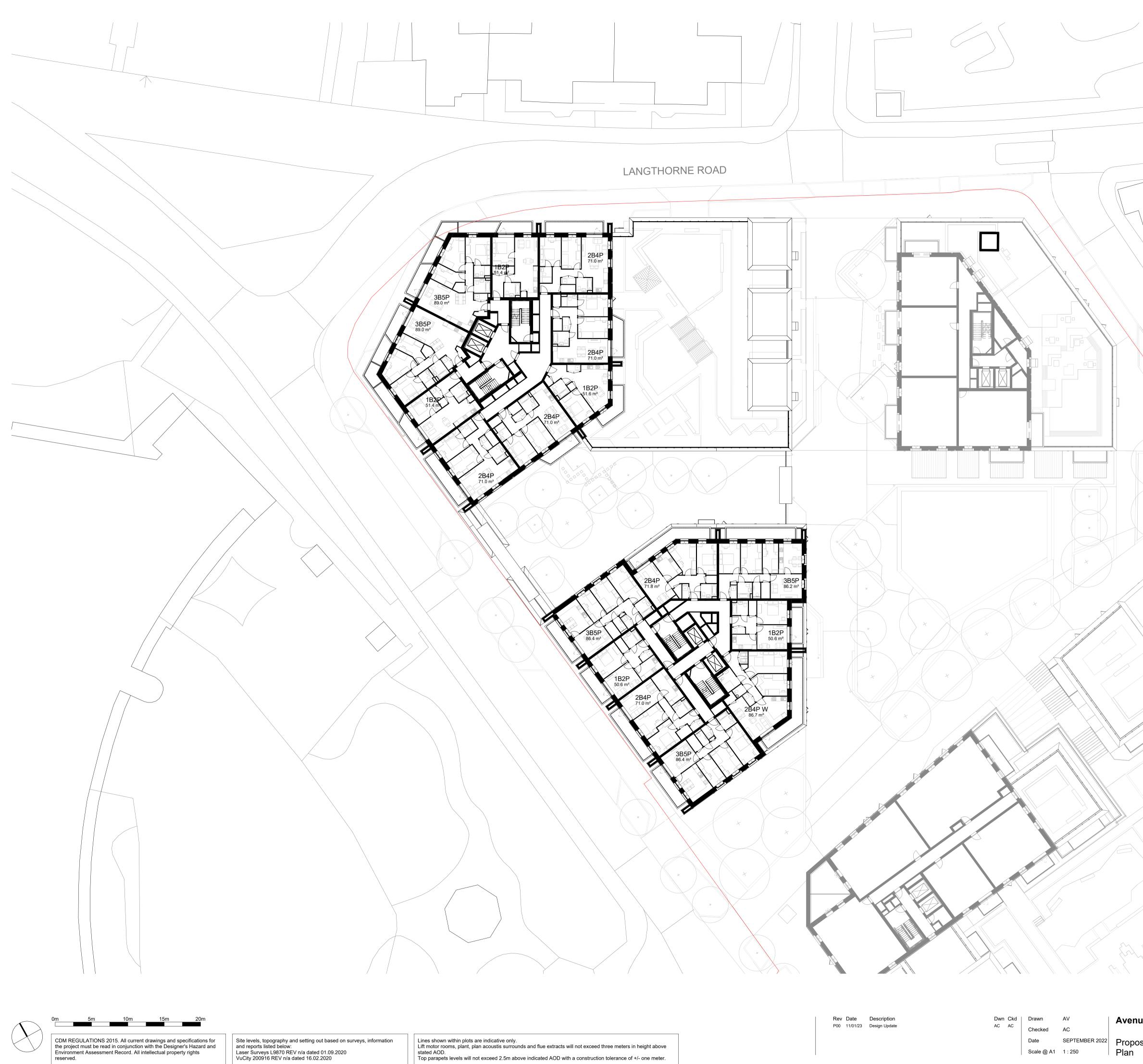
Lines shown within plots are indicative only. Lift motor rooms, plant, plan acoustis surrounds and flue extracts will not exceed three meters in height above stated AOD. Top parapets levels will not exceed 2.5m above indicated AOD with a construction tolerance of +/- one meter.
