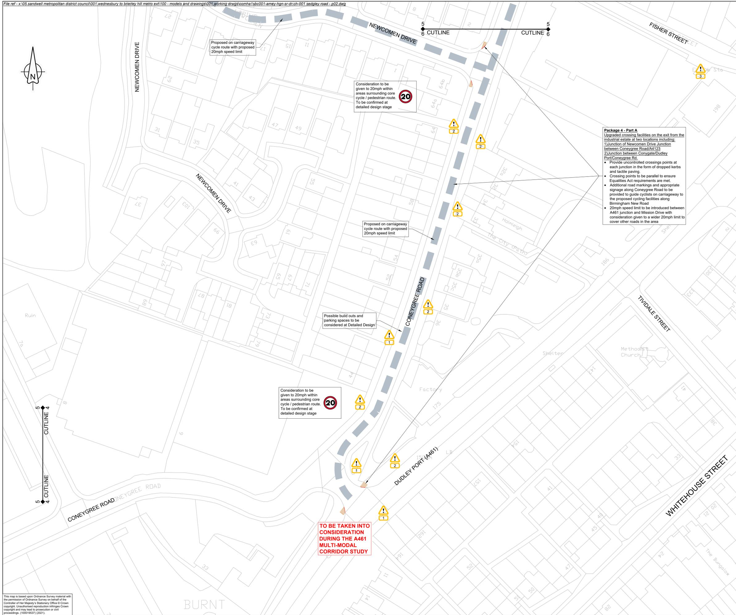
Proposed on carriageway cycle route with proposed 20mph speed limit
