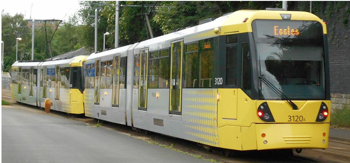
'Double' M5000 tram formation, with space at the centre unavailable to passengers
