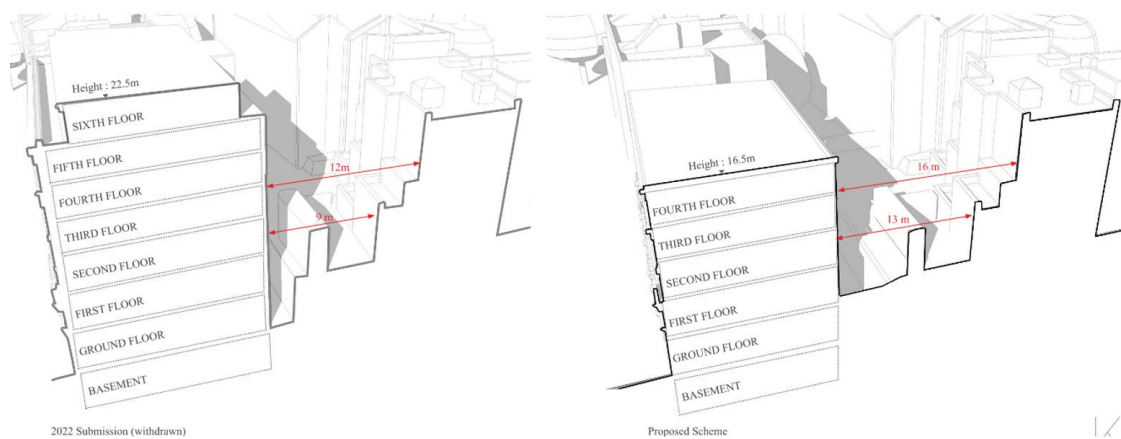
Figure 8 - Reduction in height and increased separation.
