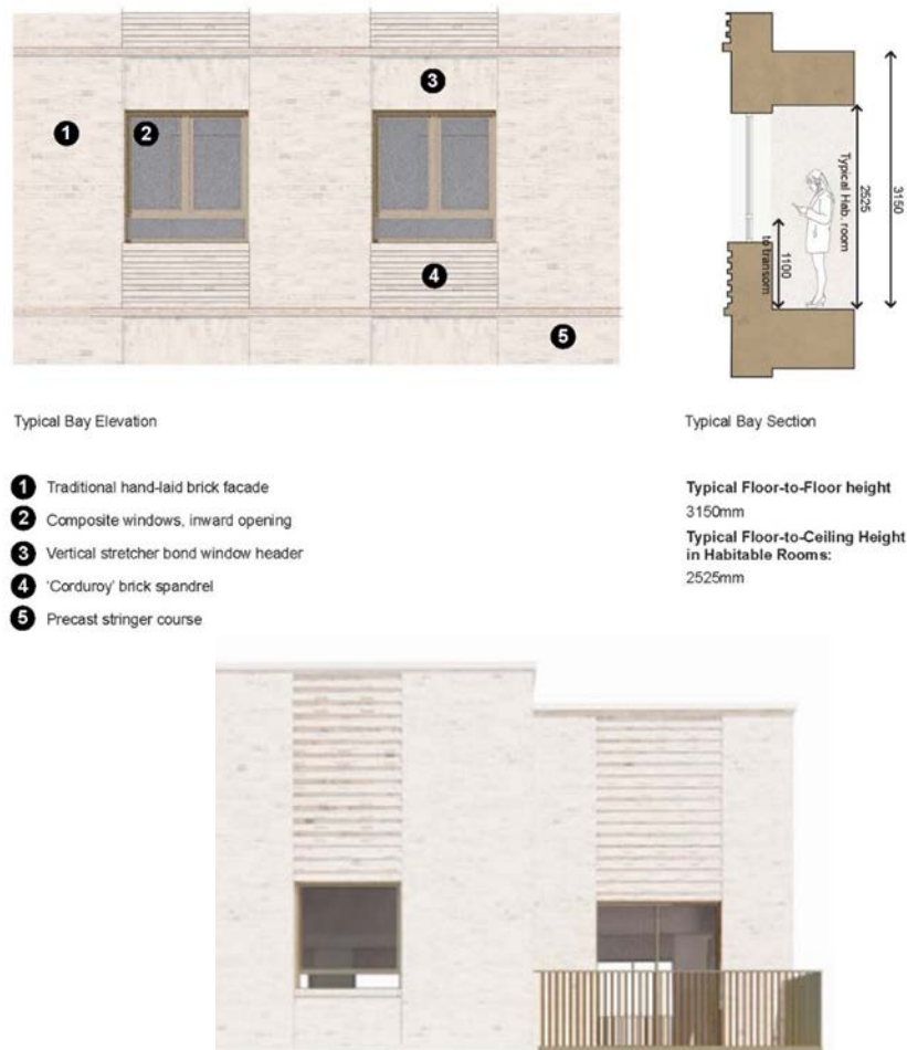
Figure 39 - B2 block typical window spandrel and crown detail (recessed alternating wite brick courses)
