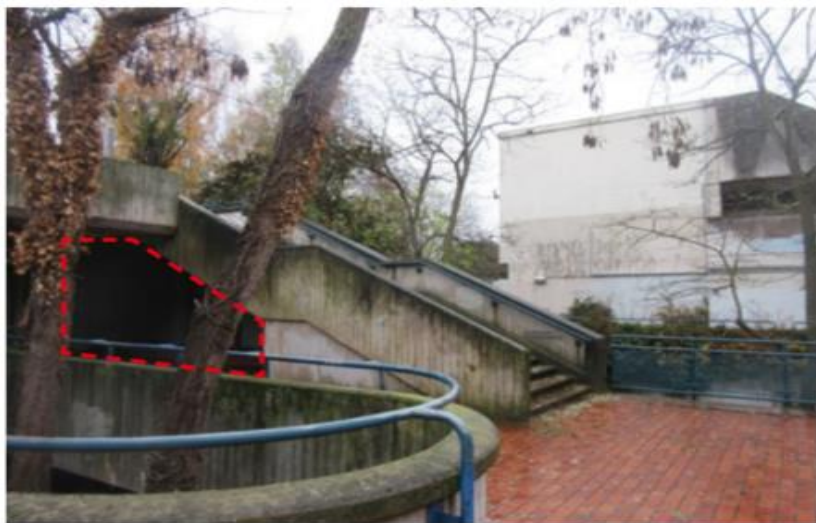
View of enclosure area below the stair. Proposed Sub-Plant Room highlighted by red dotted line
