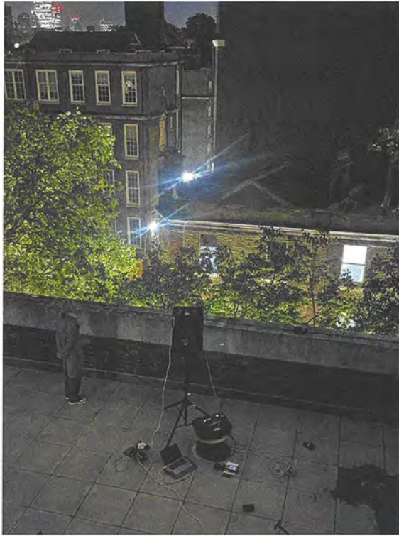
Figure 6: Source location for Level 3 terrace measurements
