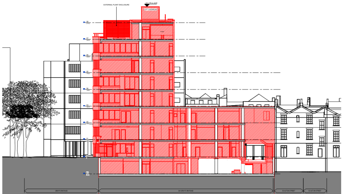
Image 3: Rear elevation (Section AA) showing the scope of demolition.
